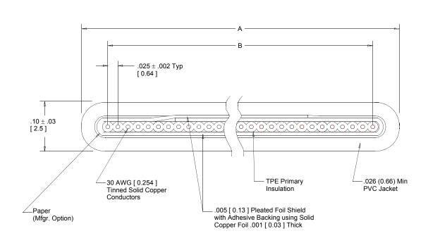
Note: Blue marking on edge of primary cable designates wire #1.
